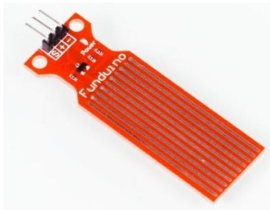
One example of the usage can be a rain detector. If the drop sensor measures a rain drop, the Arduino board could e.g. close the blinds, set off an alarm or turn on windshield wipers.
