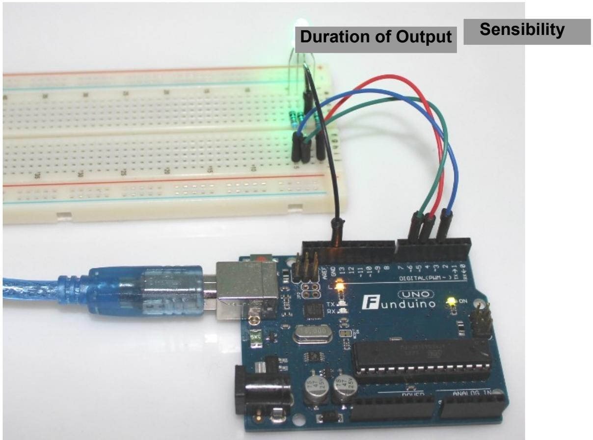
What is an RGB LED? The RGB LED is an LED that is able to shine in different colours. RGB stands for the three colours “red”, “green” and “blue”. Inside the RGB LED are three separate LEDs available, which can be turned on and off individually and shine in three different colours. That is reason behind the four contacts of the RGB LED. The longest one can be (depending on the version) the anode(+) or the cathode(-). The other contacts belong to the different colours.
