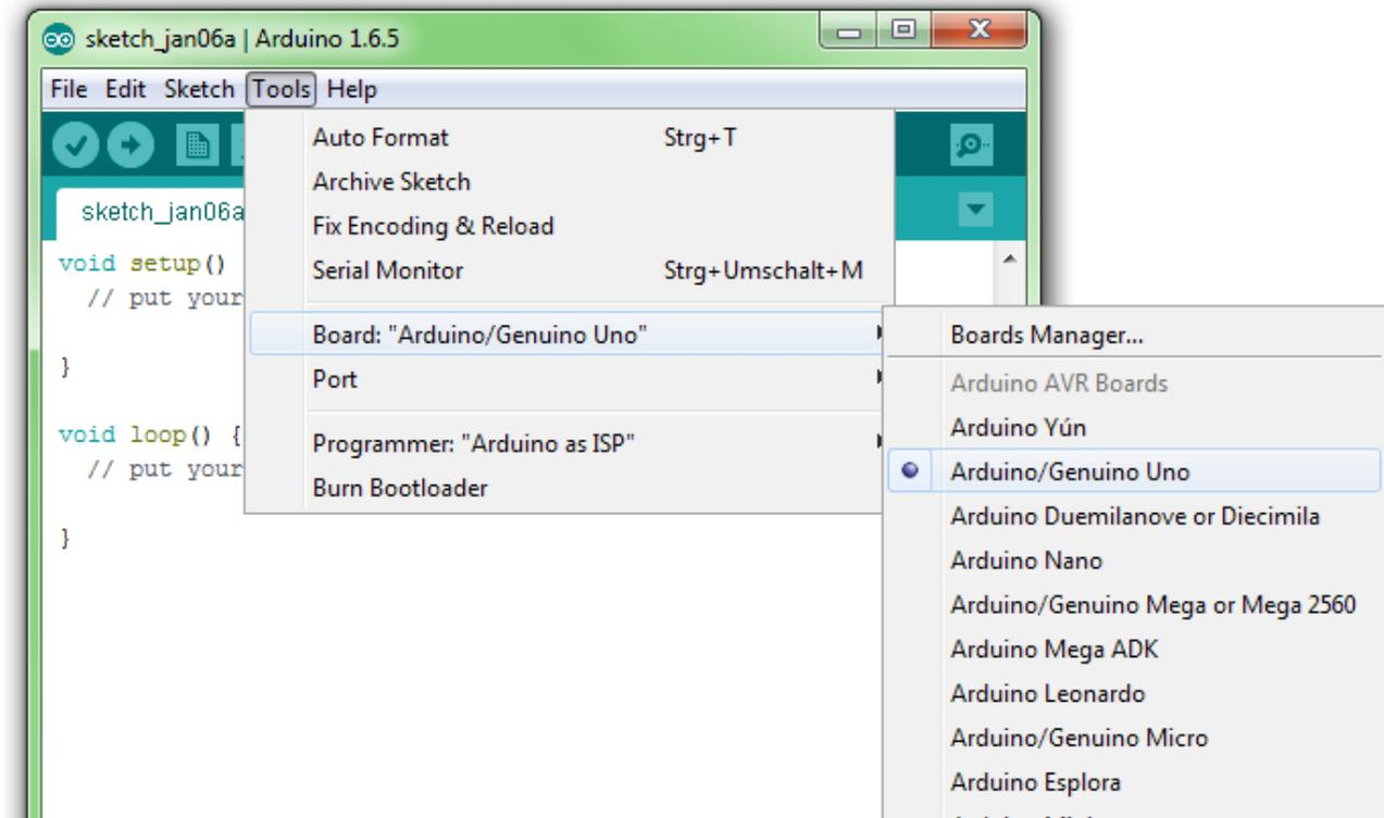
b) You have to choose the right “Serial-Port”, to let the Computer know to which port the board has been connected. That is only possible if the USB driver has been installed correctly. It can be checked this way:
