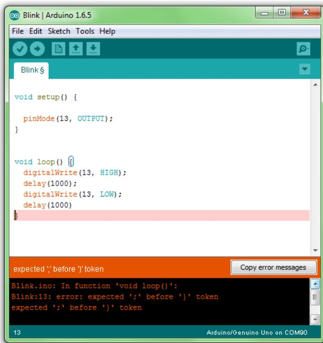
2.) There is a mistake in the sketch. For example, a word is misspelled or a bracket is missing. In the example on the left the last semicolon in the sketch is missing. In this Case the error report often starts with “expected..”. This means that the program is still expecting something that is missing.
