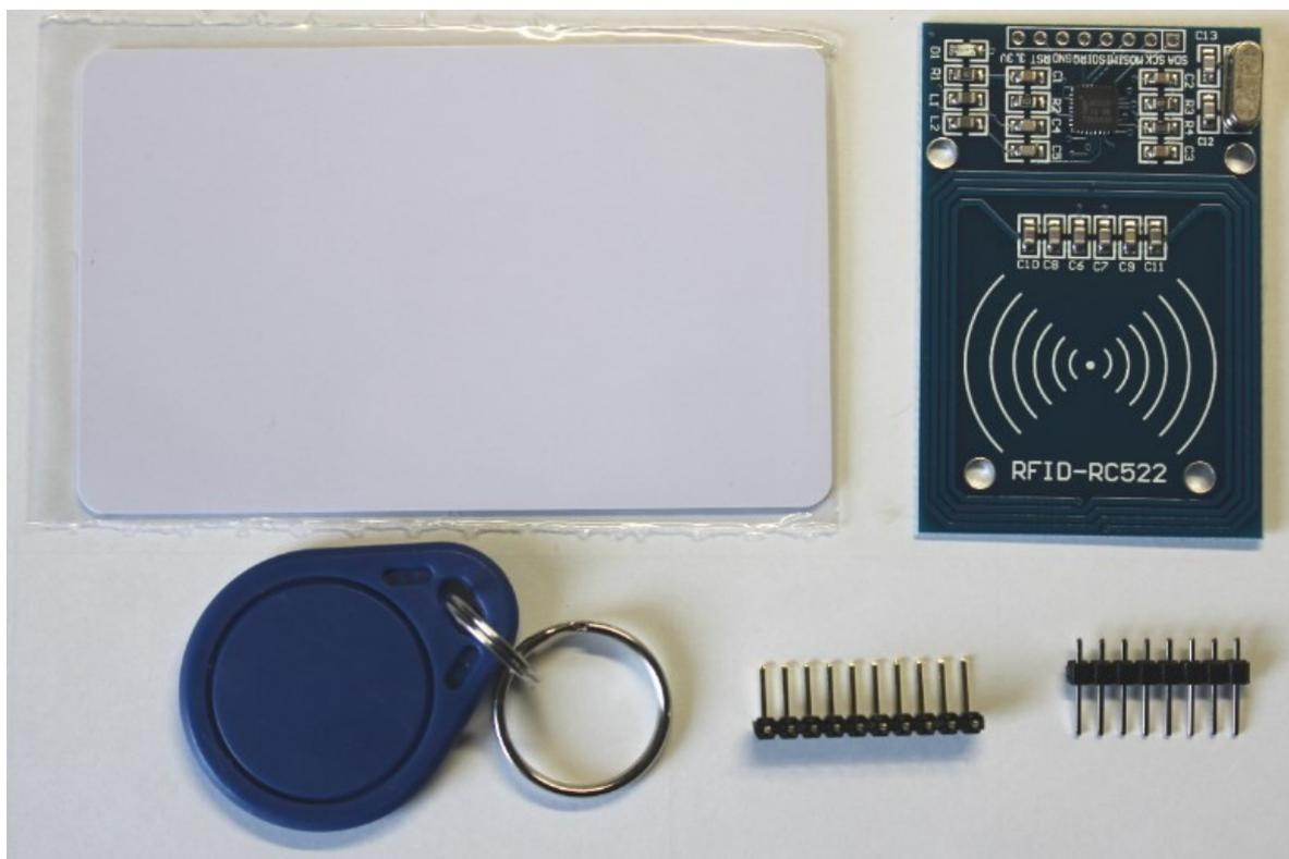
How does it work? A RFID receiver contains a small copper coil that generates a magnetic field. An RFID transmitter also includes a copper coil that picks up the magnetic field and generates an electrical voltage inside the transmitter. This voltage is used by a small electronic chip to get it to emit an electrical code by radio. The transmitter directly receives this code and processes it, so that the microcontroller is able to process the received code.
