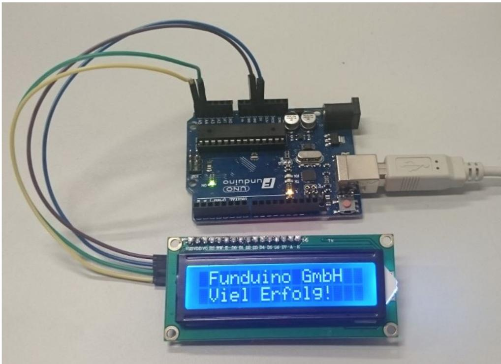
**Wiring:** The connection of the I<sup>2</sup>C LCD is very simple. The module has only four contacts. GND gets connected to GND on the Arduino, VCC to 5V on the Arduino, SDA with the analog Input A4 and SCL to the analog Input A5.
