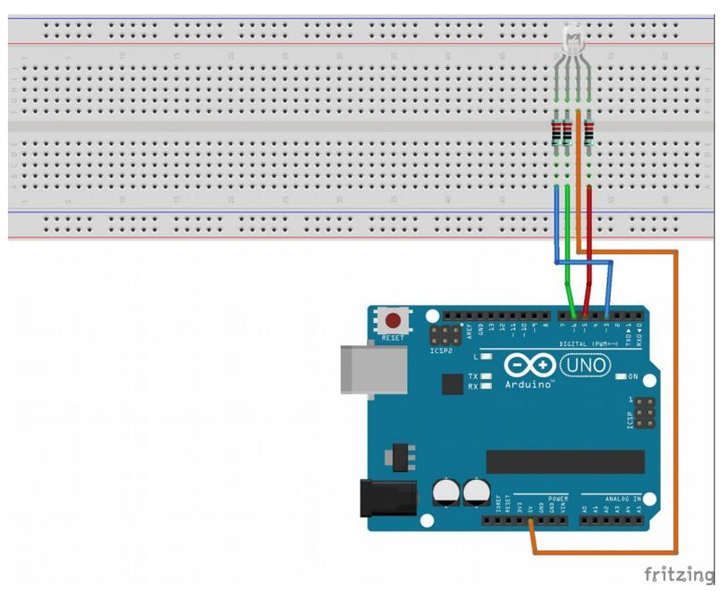
The Arduino is a digital Microcontroller. On its Outputs it only can “turn on” 5V or “turn off” 5V. But to create the different colours, the three colours of the LED have to be actuate more specific. That is the reason to use the Pulse Width Modulation. The PWM can be used on the pins with the little wave in front of the number.
